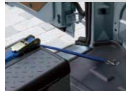
Tie-down eyes (DIN-compliant) (Standard)
