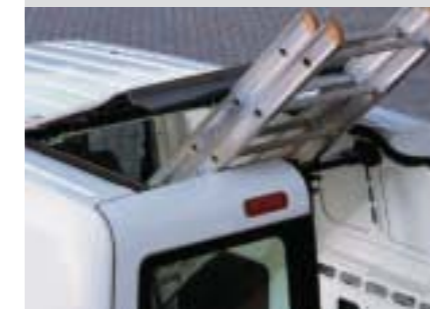
Rear roof flap Enables long or awkward loads to be safely carried. (Option on SWB with cargo doors)
