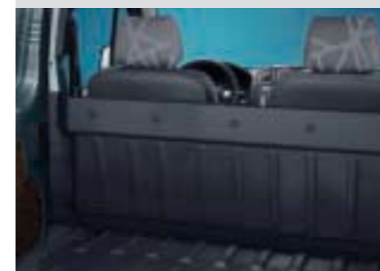
Tie-down eyes (DIN-compliant) (Standard)
